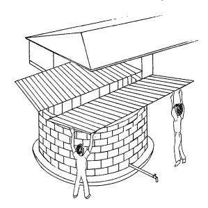
Depending on local traditional building practice, circular tanks are made with blocks of con crete or sandcrete; sun-dried, kiln-dried and adobe bricks; or masonry (natural stone). The inside is always plastered with cement mortar. The outside may also be plastered.
